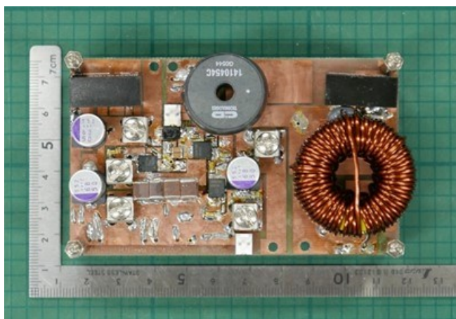
Fig. 23. Photograph of 240-W prototype.
