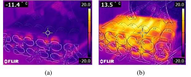
Fig. 16. Temperature distributions (a) before heating and (b) after heating for 60 minutes.
