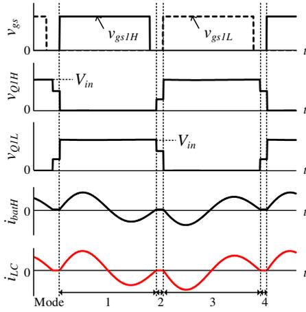
Fig. 8. Key operation waveforms in ac heating mode.
