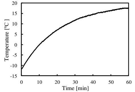
Fig. 15. Temperature evolution of the LIB surface.
