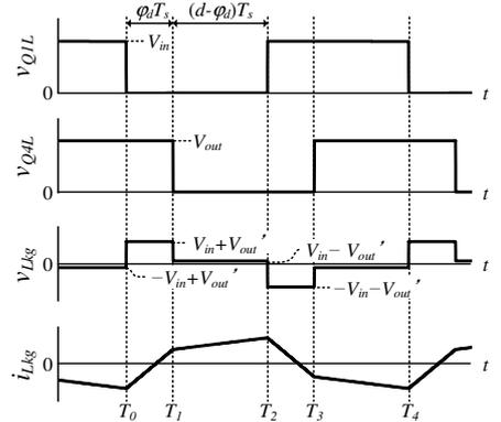
Fig. 11. Key operation waveforms in power transfer mode.
