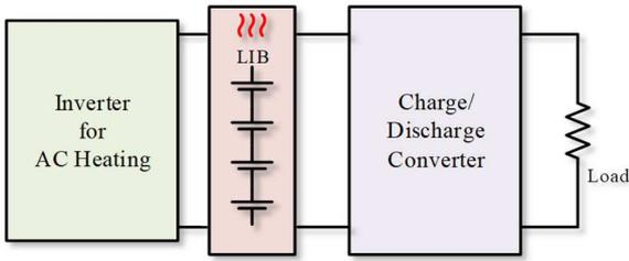
Fig. 4. LIB system using ac heating techniques.
