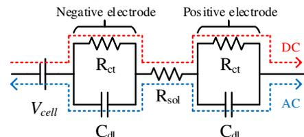
Fig. 3. Current flow directions at LIB using internal heating techniques.
