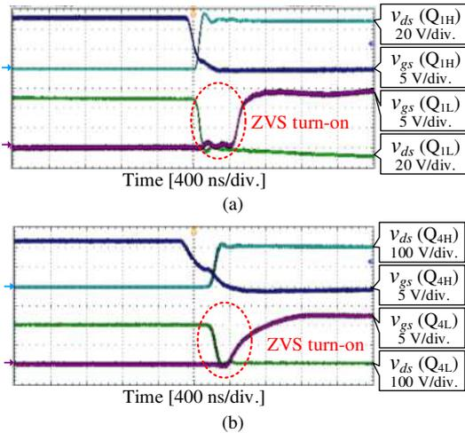
Fig. 18. ZVS waveforms at 300 W in power transfer mode. (a)  $Q_{1L}$  turn-on. (b)  $Q_{4L}$  turn-on.
