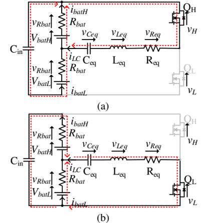
Fig. 10. Equivalent circuits in ac heating mode. (a) Mode 1 and (b) Mode 3.
