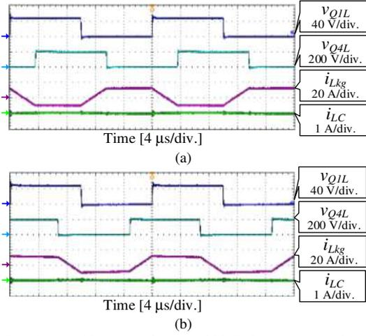
Fig. 17. Measured key waveforms at 300 W in power transfer mode. (a) The discharge operation. (b) The charge operation.
