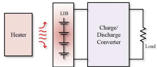
Fig. 2. LIB system using external heating techniques.
