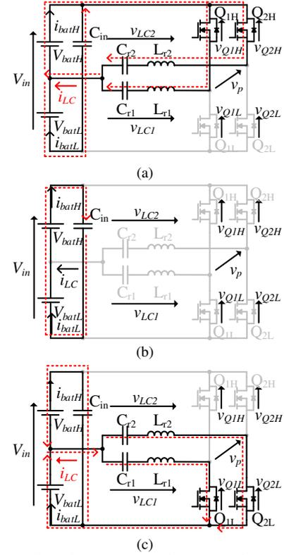
Fig. 9. Current flow directions in ac heating mode. (a) Mode 1, (b) Mode 2 and 4, and (c) Mode 3.
