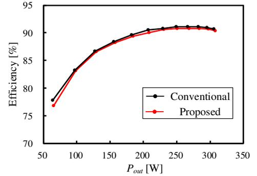
Fig. 20. Measured power conversion efficiencies.
