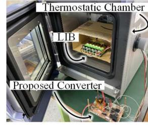
Fig. 13. Experimental platform using thermostatic chamber for LIB heating.
