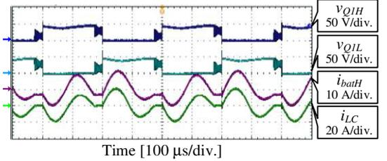
Fig. 14. Measured key waveforms in ac heating mode.
