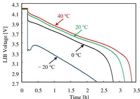
Fig. 1. Discharge characteristics of the LIB with C/3 rate at four temperatures.
